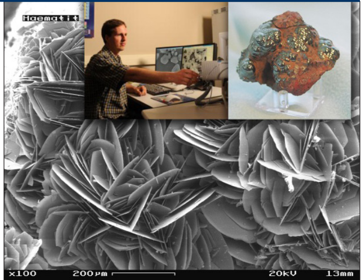
Hematite in a Scanning Electron Microscope, Magnification 100X (Wikipedia)
